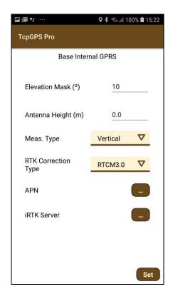
Figure 3. Base GPRS working mode
