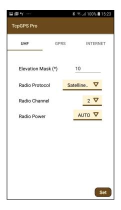
Figure 4. Rover UHF working mode
