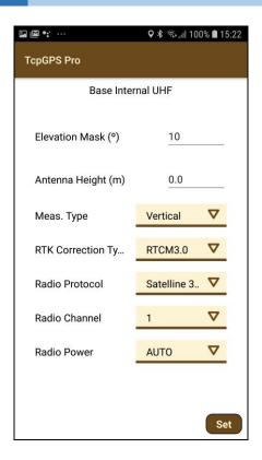
Figure 2. UHF Base working mode
