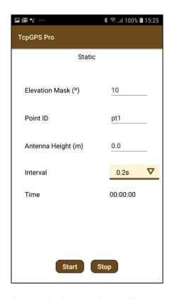
Figure 7. Static recording configuration
