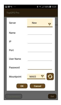
Figure 9. NTRIP configuration
